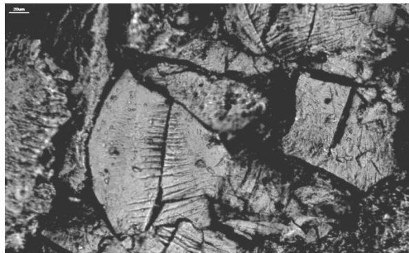
Figure 4 – Brittle and plastic deformation in a single coal particle
